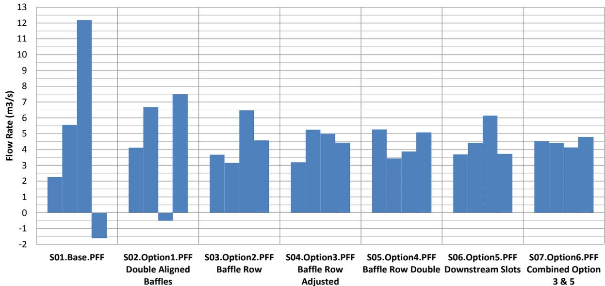
Figure 3.21: PFF – Mean Flow in Channels
