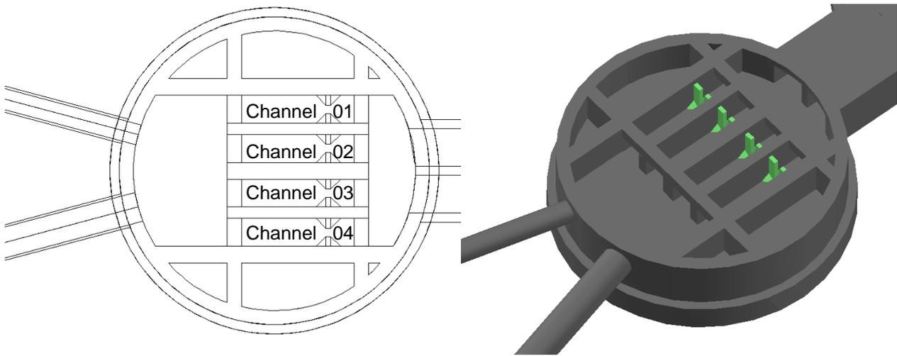
Figure 3.15: Baffled Option 5 – Downstream Slots
