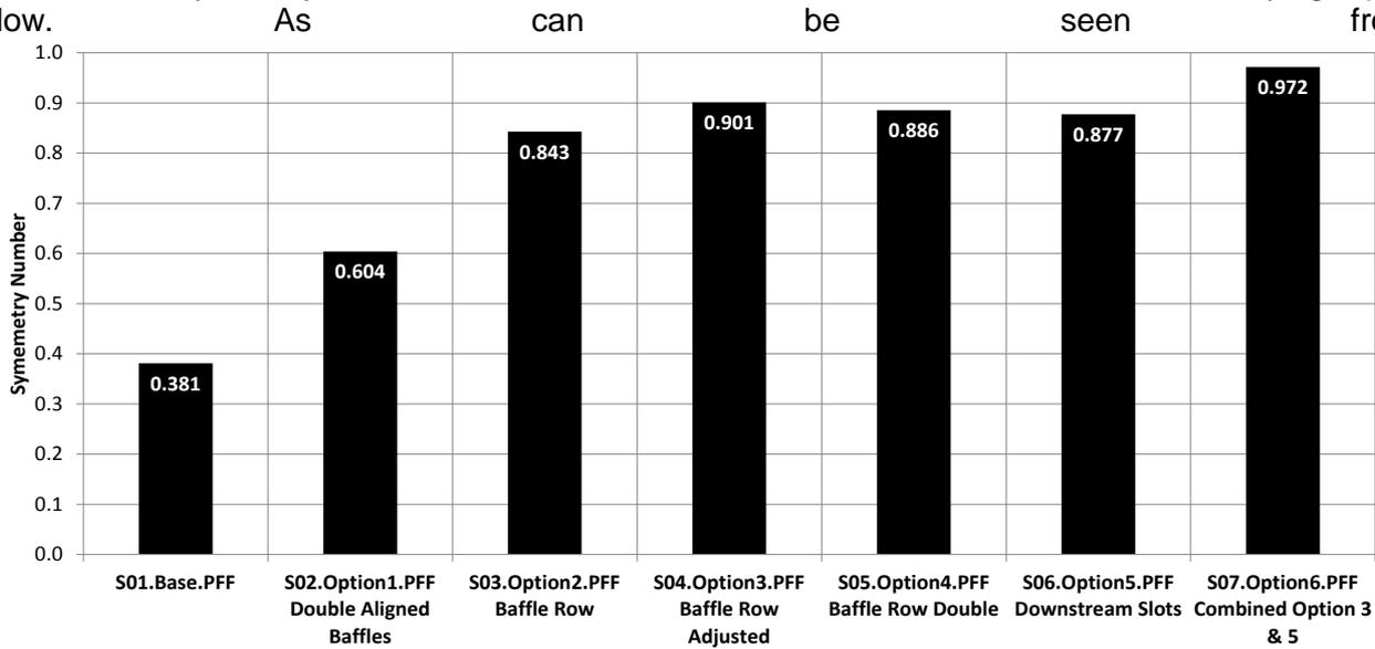
Figure 3.25 below, Option 6 achieves the most symmetrical flows followed by Option 3 and Option 4 which achieving the next highest symmetry coefficients and also meeting the acceptance criteria of no greater than +/- 33% of the average flow through any channel.
