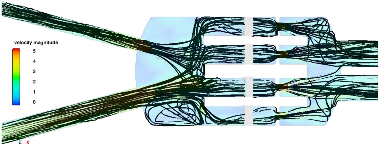
Figure 3.17: S06.Option5.PFF – Plan View - Streamlines
