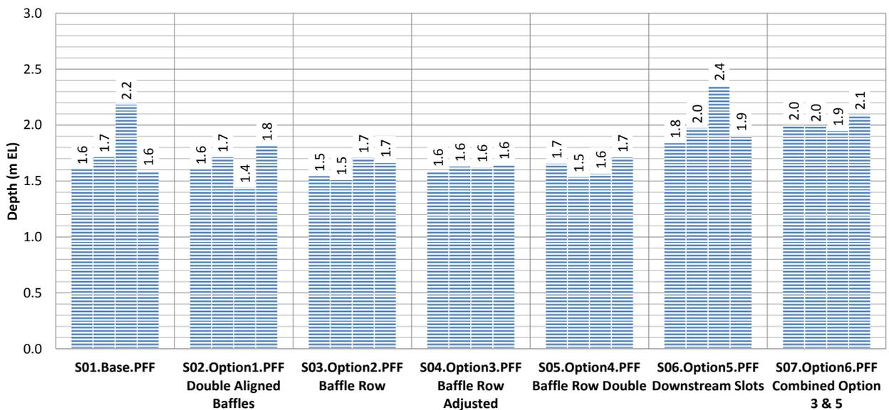
Figure 3.24: PFF – Mean Flow Depth in Channels
