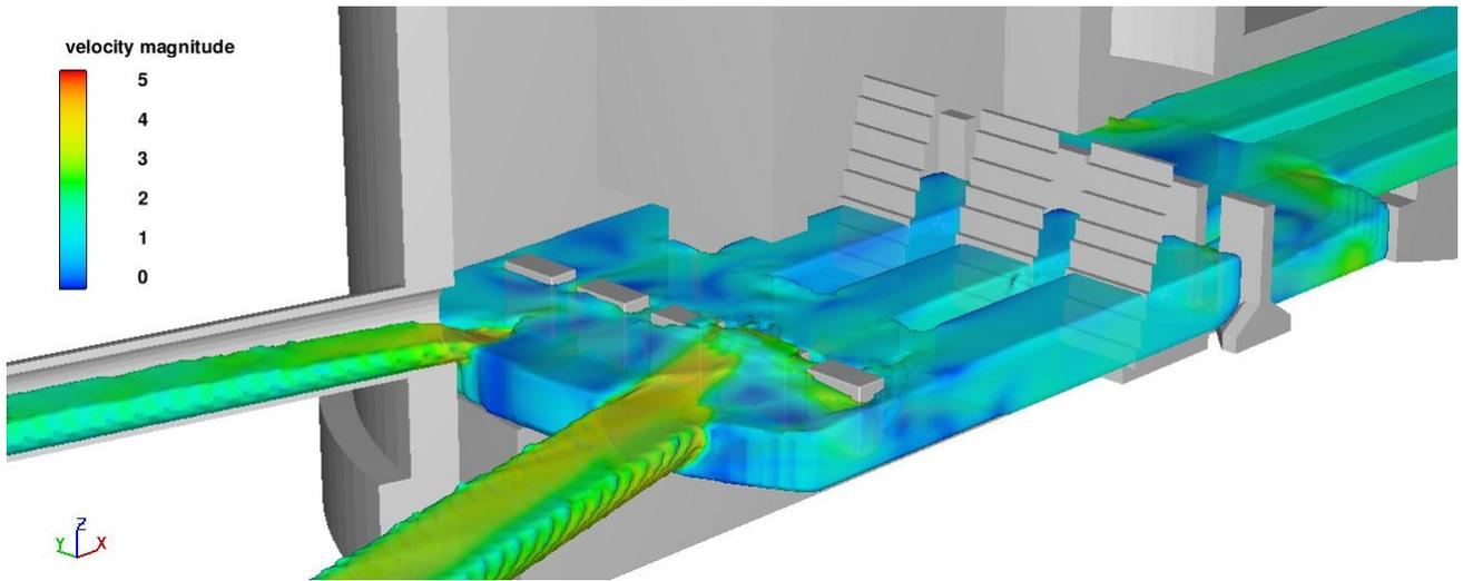
Figure 3.19: S07.Option6.PFF - 3D View - Surface Velocity (m/s)
