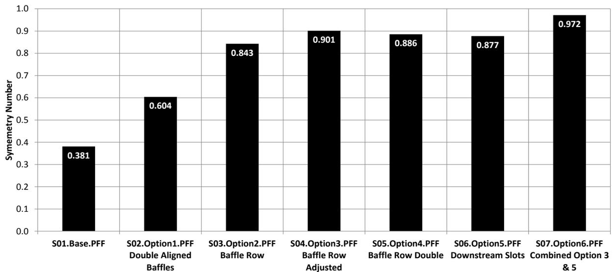
Figure 3.25: PFF – Flow Symmetry Coefficient per geometry option
