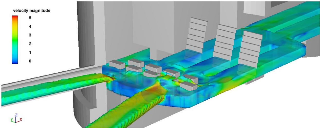
Figure 3.13: S05.Option4.PFF - 3D View - Surface Velocity (m/s)the flow distribution.
