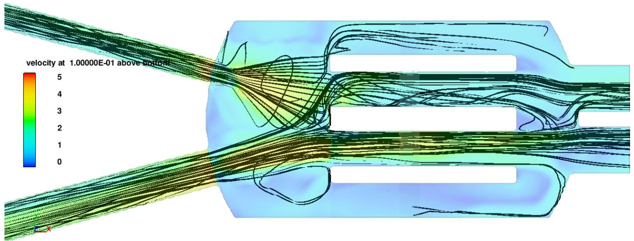
Figure 3.2: S01.Base.PFF – Plan View – Streamlines
