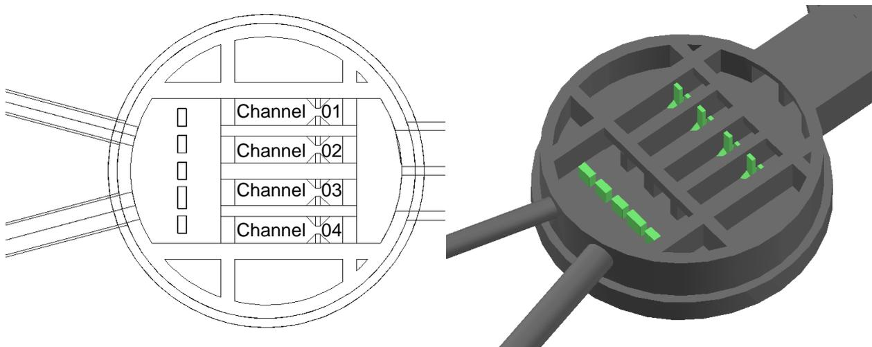
Figure 3.18: Baffled Option 6 – Baffle Row and Downstream Slots
