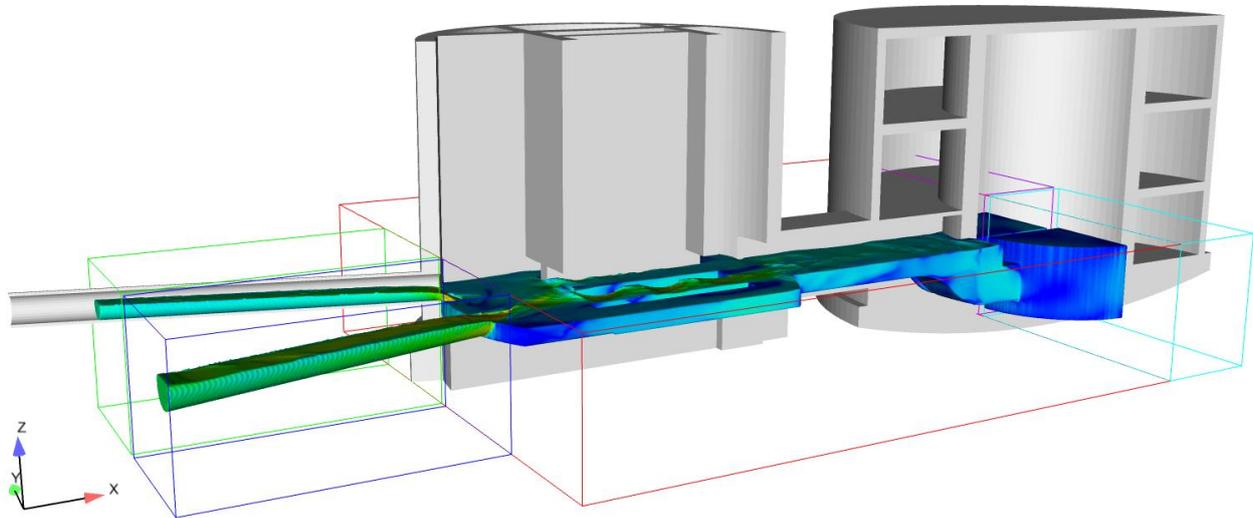
Figure 2.1: Model Setup showing geometry sectioned, computational mesh blocks and flows
