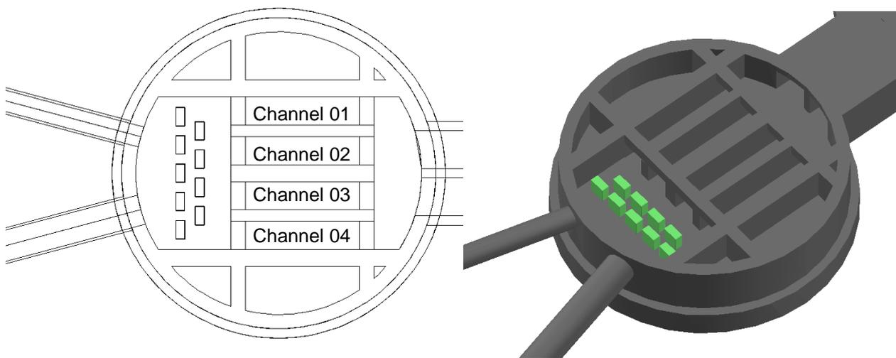
Figure 3.12: Baffled Option 4 – Double Baffle Row
