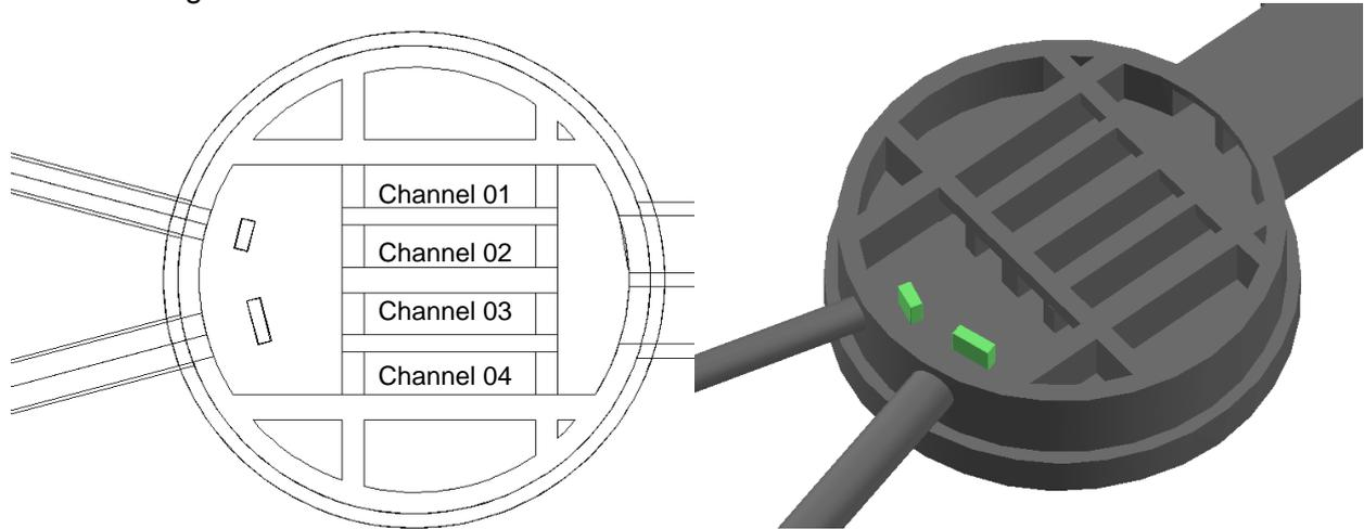
Figure 3.3: Baffled Option 1 – Double aligned baffles
