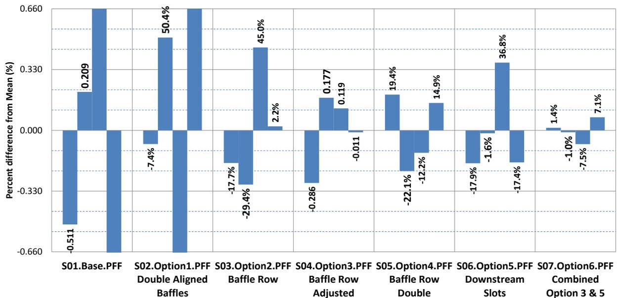
Figure 3.22: PFF – Percent Difference from Mean Flow in Channels
