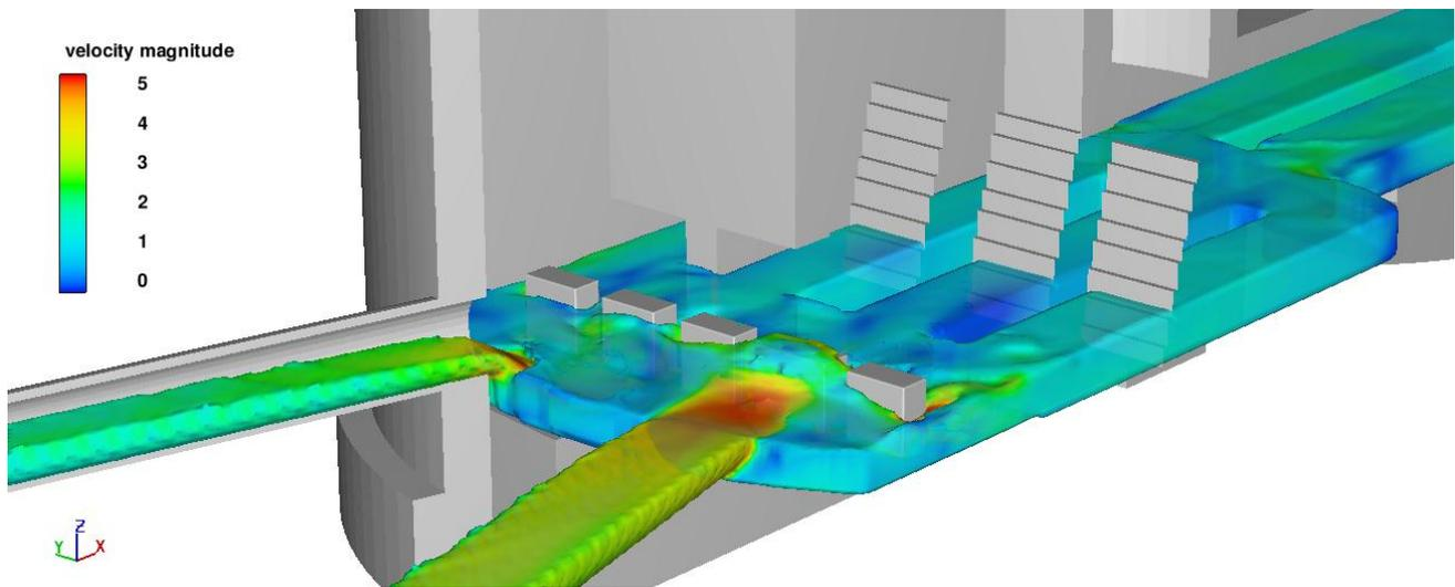
Figure 3.10: S04.Option3.PFF - 3D View - Surface Velocity (m/s)
