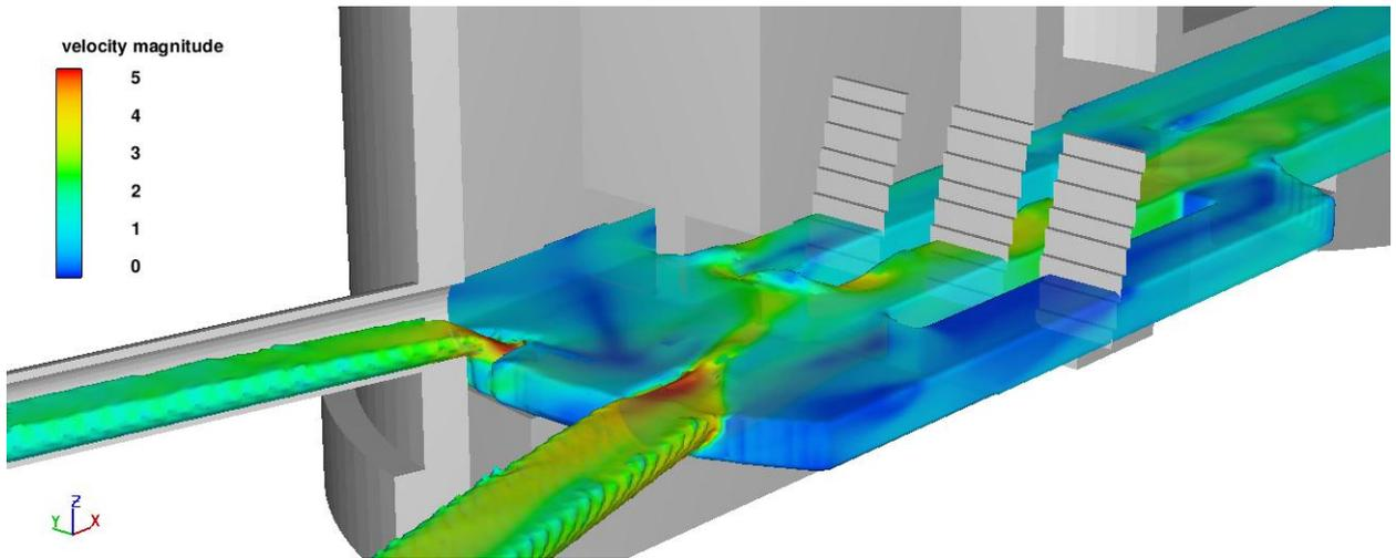
Figure 3.1: S01.Base.PFF - 3D View – Surface velocity (m/s)
