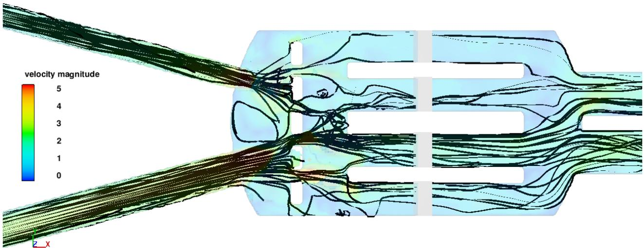
Figure 3.8: S03.Option2.PFF – Plan View – Streamlines
