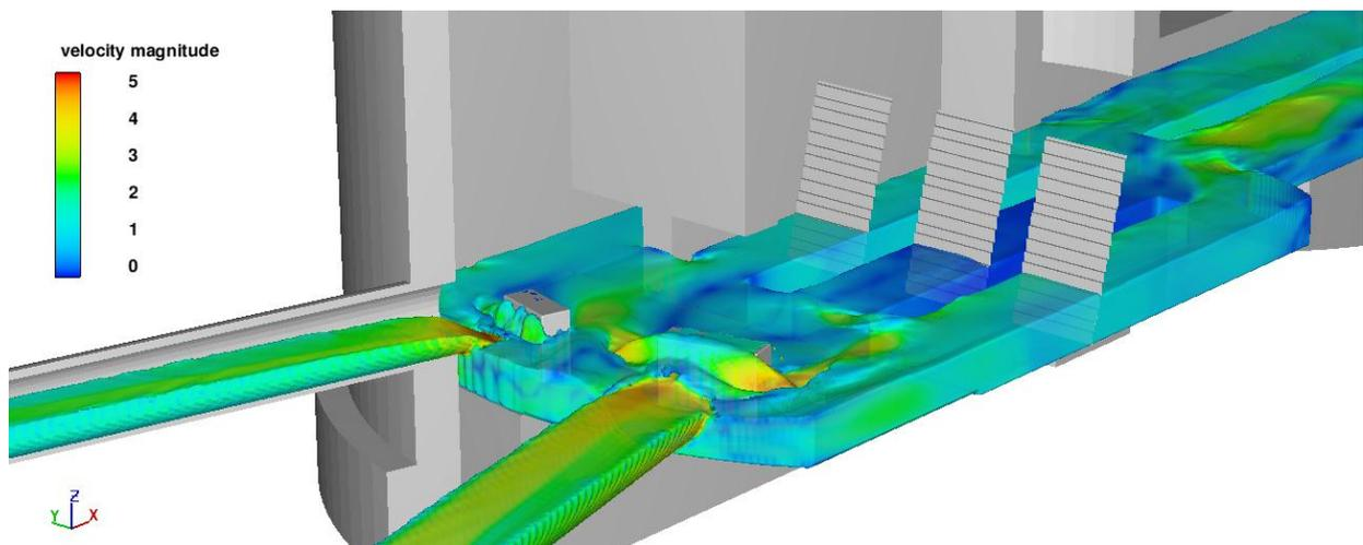
Figure 3.4: S02.Option1.PFF – 3D View - Surface Velocity (m/s)
